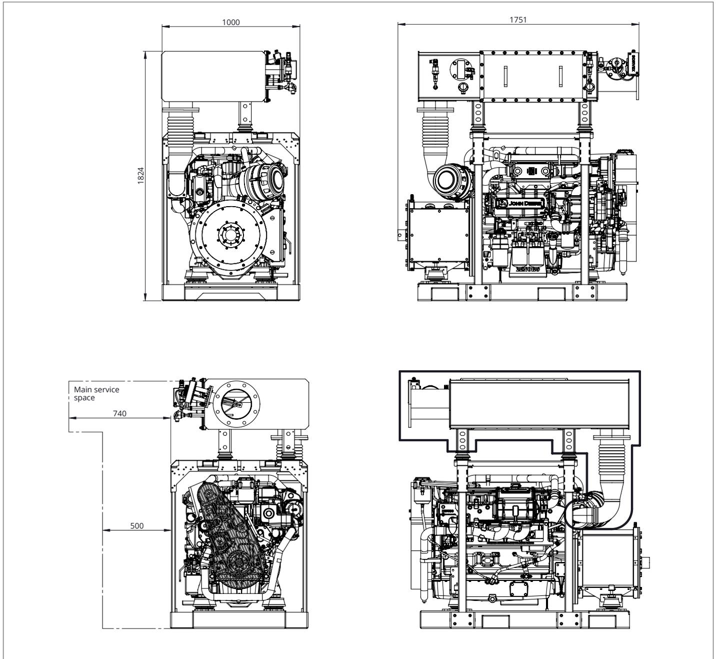
NOTE: Generator sets to be installed above waterline. If not consult factory.
