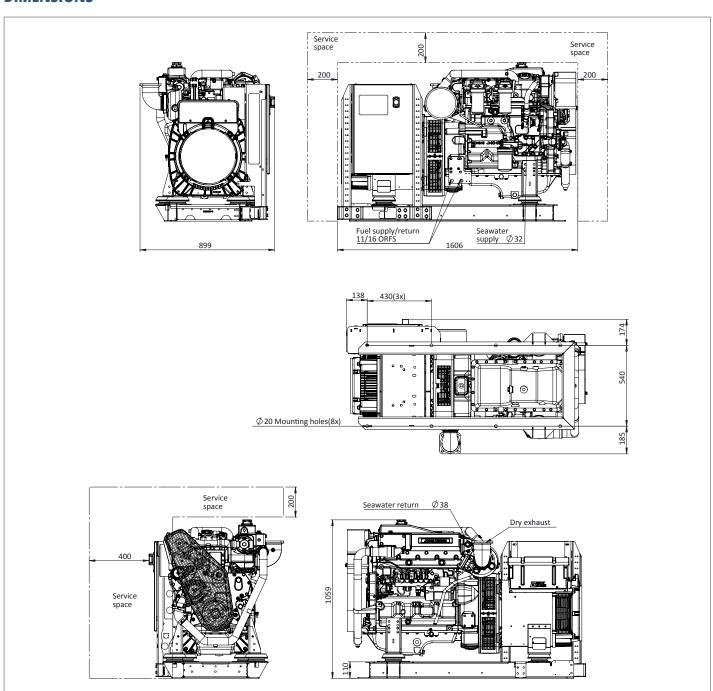
$\label{eq:NOTE: Generator sets to be installed above waterline. If not consult factory. \\$
