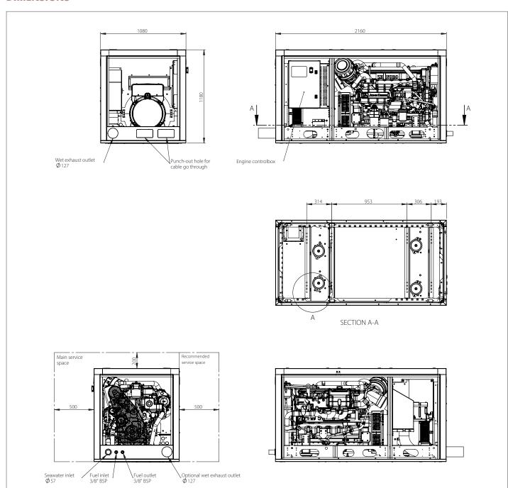
NOTE: Generator sets to be installed above waterline. If not consult factory. Minimum space required to remove air panels 200 mm, non air panels 80 mm. This drawing is provided for reference only and is not intended for installation purpose. Contact us either your local distributor for detailed information.
