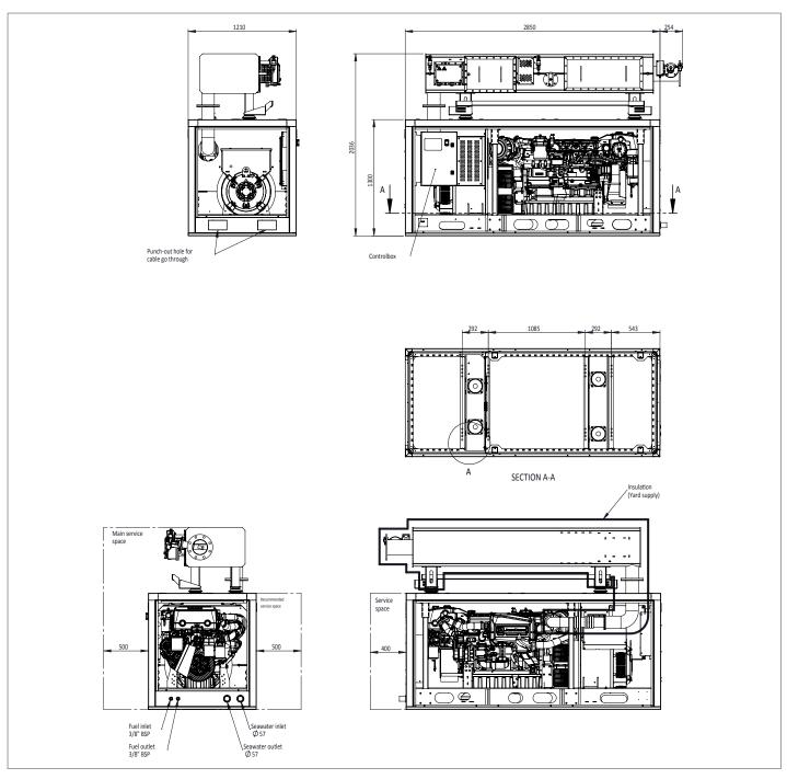
NOTE: Generator sets to be installed above waterline. If not consult factory. Minimum space required to remove air panels 200 mm, non air panels 80 mm. This drawing is provided for reference only and is not intended for installation purpose. Contact us either your local distributor for detailed information.
