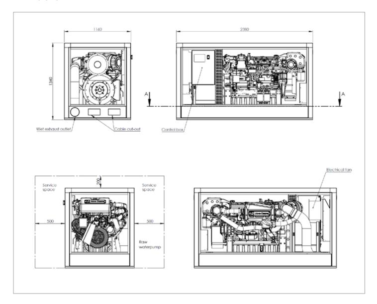
NOTE: Generator sets to be installed above waterline. If not consult factory. Minimum space required to remove air panels 150 mm, non air panels 80 mm. This drawing is provided for reference only and is not intended for installation purpose. Contact us either your local distributor for detailed information.
