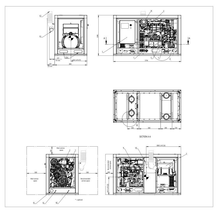
NOTE: Generator sets to be installed above waterline. If not consult factory. Minimum space required to remove air panels 150 mm, non air panels 80 mm. This drawing is provided for reference only and is not intended for installation purpose. Contact us either your local distributor for detailed information.
