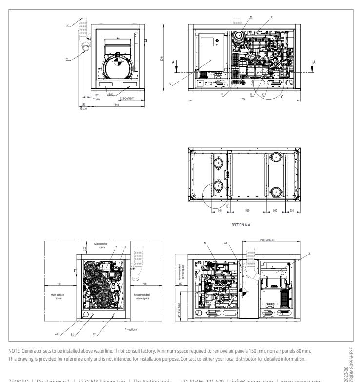
NOTE: Generator sets to be installed above waterline. If not consult factory. Minimum space required to remove air panels 150 mm, non air panels 80 mm. This drawing is provided for reference only and is not intended for installation purpose. Contact us either your local distributor for detailed information.
